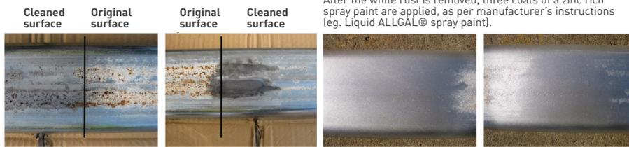
Figure 2: White rust repair using Vinegar and nylon scourer
